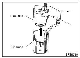
16. Separate the fuel filter and chamber.
