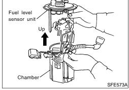
14. Pull up the fuel level sensor unit from chamber.
