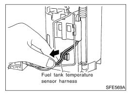
9. Pull out the fuel tank temperature sensor harness.
