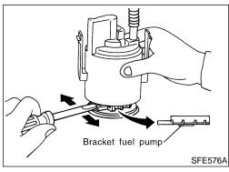
17. Remove fuel pump bracket, then pull out from the fuel filter.
